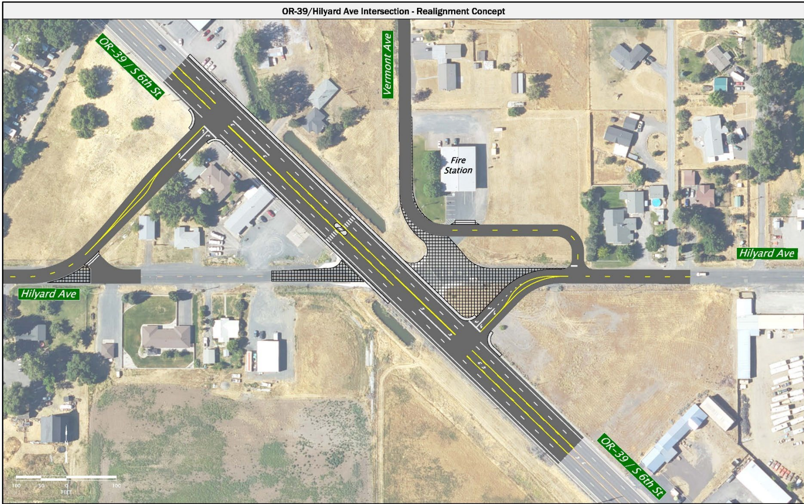
Figure 6 OR 39/Hilyard Ave Realignment Concept Solution ID #5
