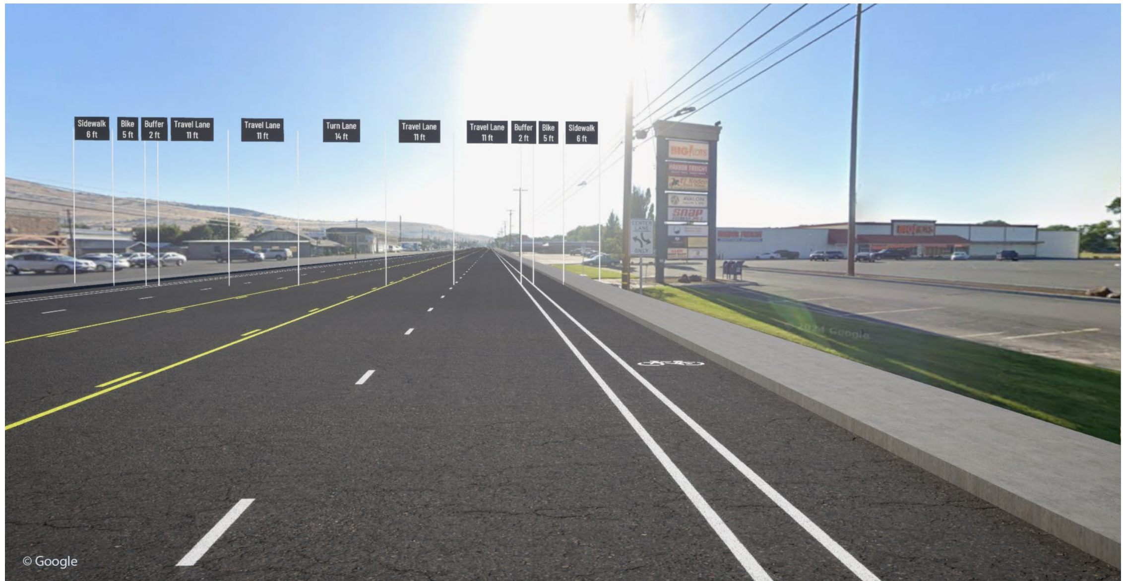
Figure 9 OR 39: Altamont Dr to Summers Lane Typical Cross Section – Solution ID #8
