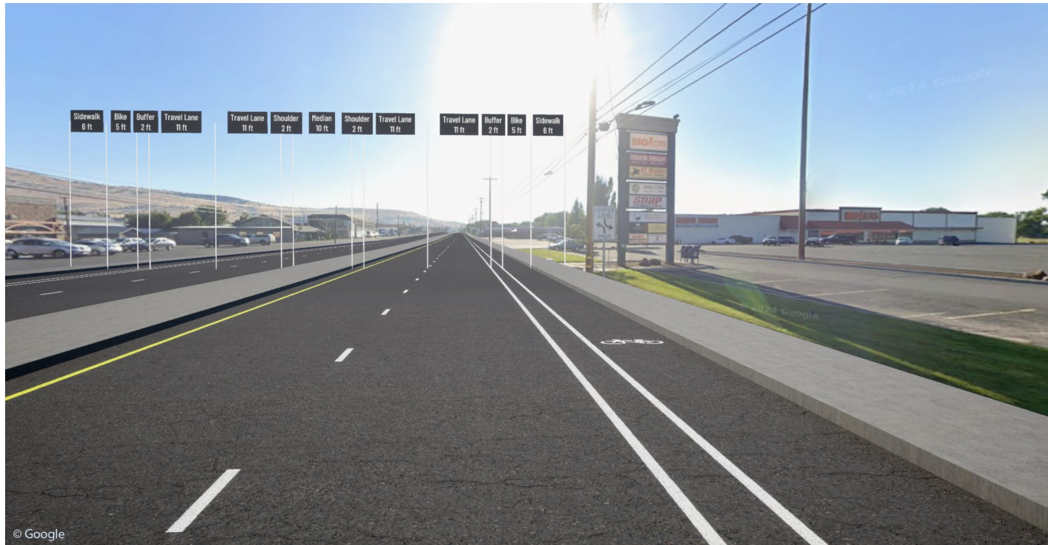
Figure 10 OR 39: Altamont to Summers Lane Typical Cross Section – Solution ID #9
