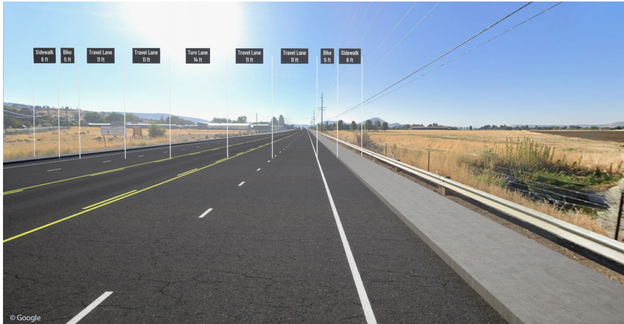
Figure 13: OR 39: Hilyard to OR 140 Typical Cross Section – Solution ID #12
