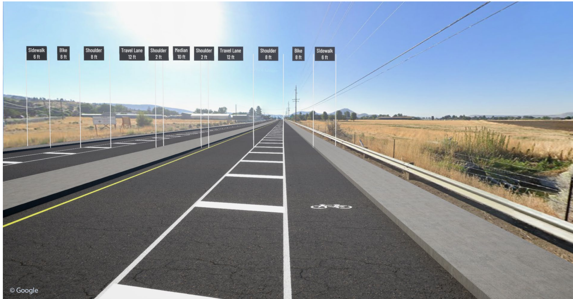
Figure 14 OR 39: Hilyard to OR 140 Typical Cross Section – Solution ID #13
